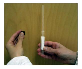
3. Place the straw in the your mouth with the breath collection tube at the end of the straw. Take a full breath and exhale through the straw directly into the tube. The breath should not be forced.
